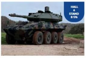
ammunition magazines. The 105/52 mm gun produced by Leonardo is fully equivalent to the L7: it has however a higher safety coefficient. thanks to the use of advanced materiel. The muzzle brake is of the pepperbox type, like that of the 120 mm gun but with an added baffle.
